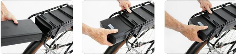
The battery automatically locks into the bike when fully inserted in the battery holder. The locking mechanism is spring loaded and unlocks when the key is turned to the open position, allowing the battery to slide out. The battery must be locked when riding or it may fall out. The key does not have to be in to operate the bike.
